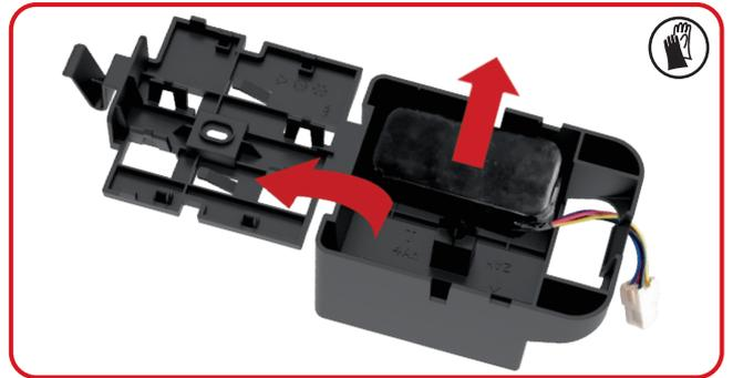
6. Put the battery box back in its position and plug the connectors. Refit the sheet metal.
