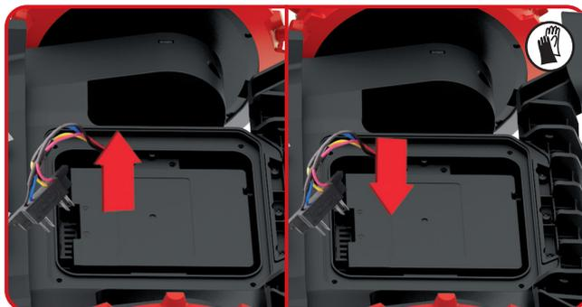
5. Refit the sheet metal. Place the cover back in its position and tighten the screws.
