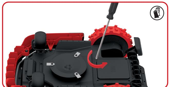
3. Remove the screws on the sheet metal.
