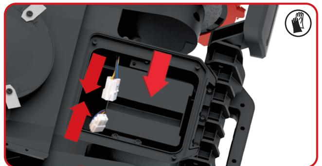
7. Place the cover back in its position and tighten the screws.
